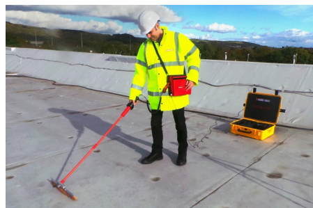
▲ HIGH VOLTAGE DISCHARGE TEST
