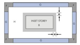
A further zone (shadow zone) around the base of the inset storey should be included. This shadow zone should extend by a distance of ' $\mathbf{e}$ ' from the base of the inset storey. The dimension ' $\mathbf{e}$ ' also represents the scaling length of the inset storey.
