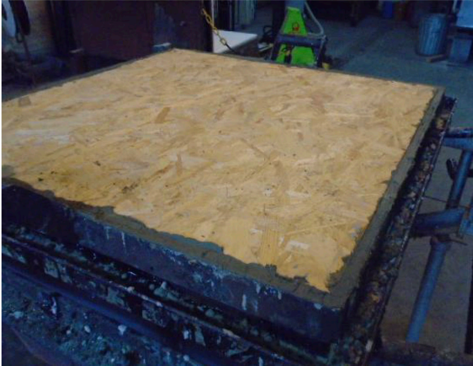
Figure 12- OSB board test 1 as installed prior to testing.
