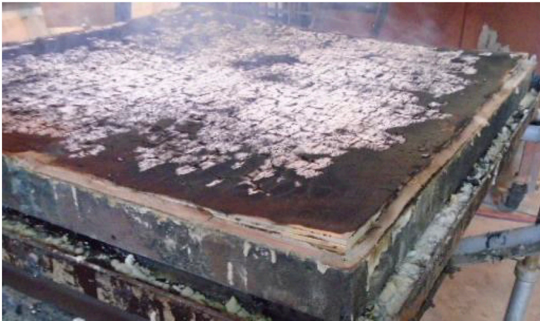
Figure 7- showing edge seal failure.
