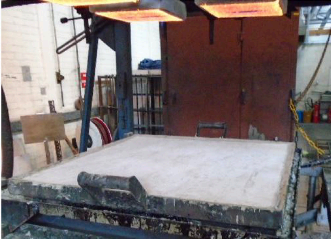
Figure 19- Test specimen 1 at end of 60 minute test.
