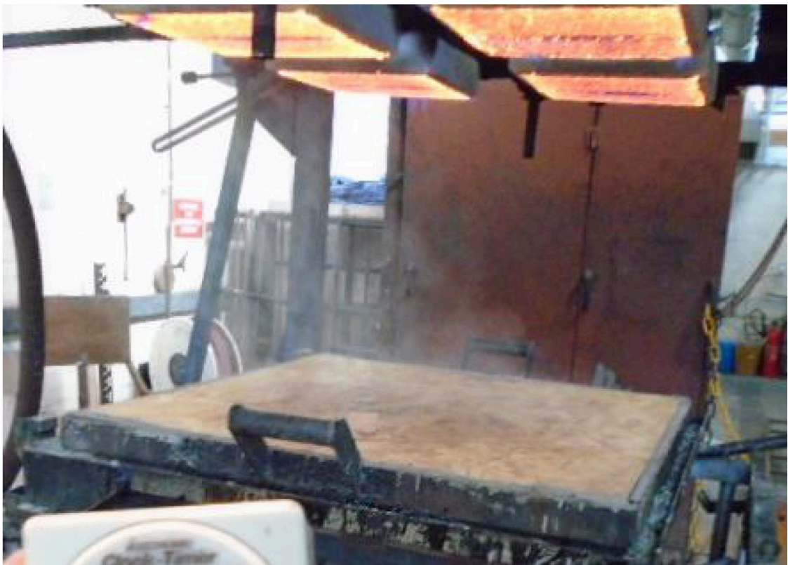
Figure 15- Test specimen at 4:25 minutes, prior to ignition.
