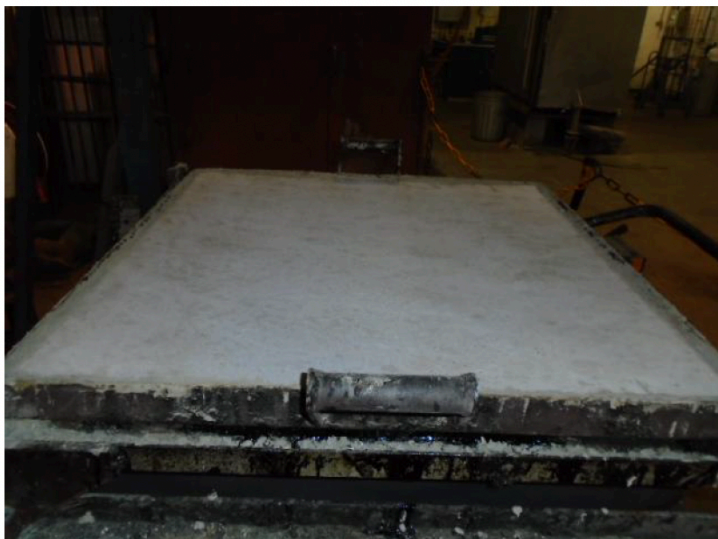
Figure 21- Test specimen 2 at end of 60 minute test.
