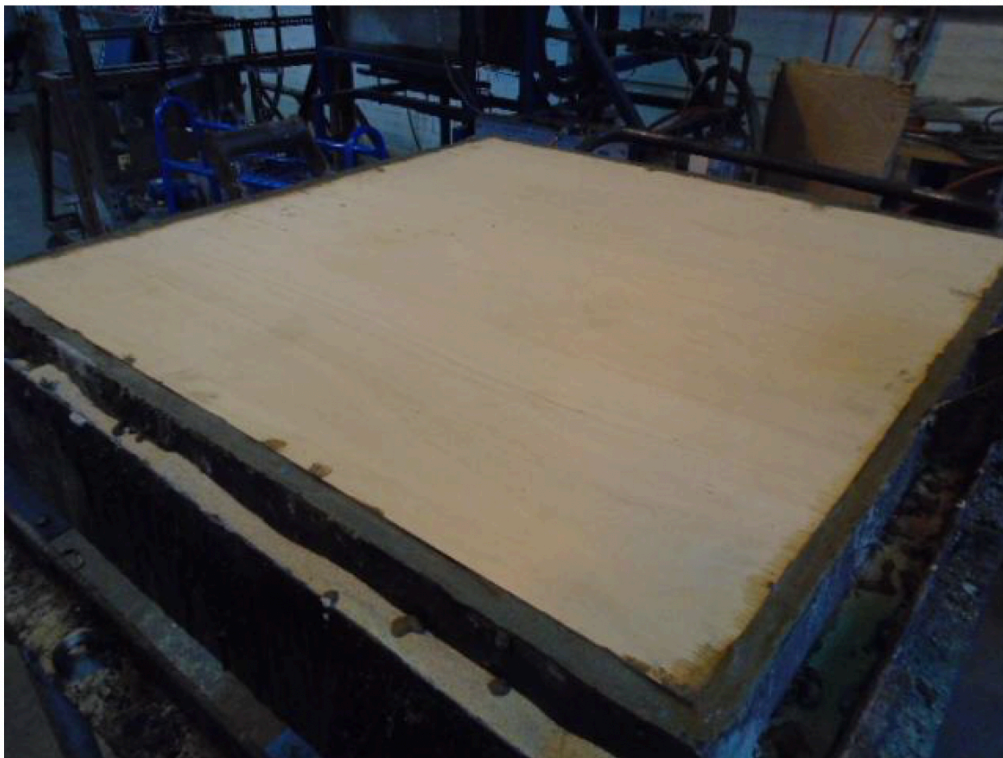
Figure 3- plywood specimen as installed prior to testing.
