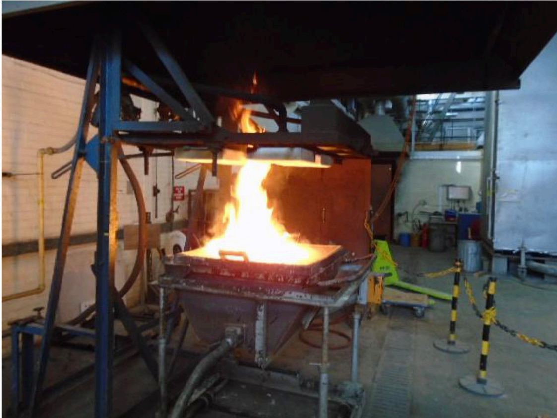
Figure 14- Test 1 immediately before test stopped at 6:30 minutes due to flames threatening gas pipes above test rig.
