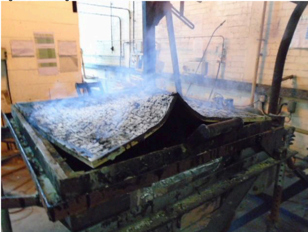
Figure 10- showing severe warping of test specimen 2 at approximately 36 minutes.
