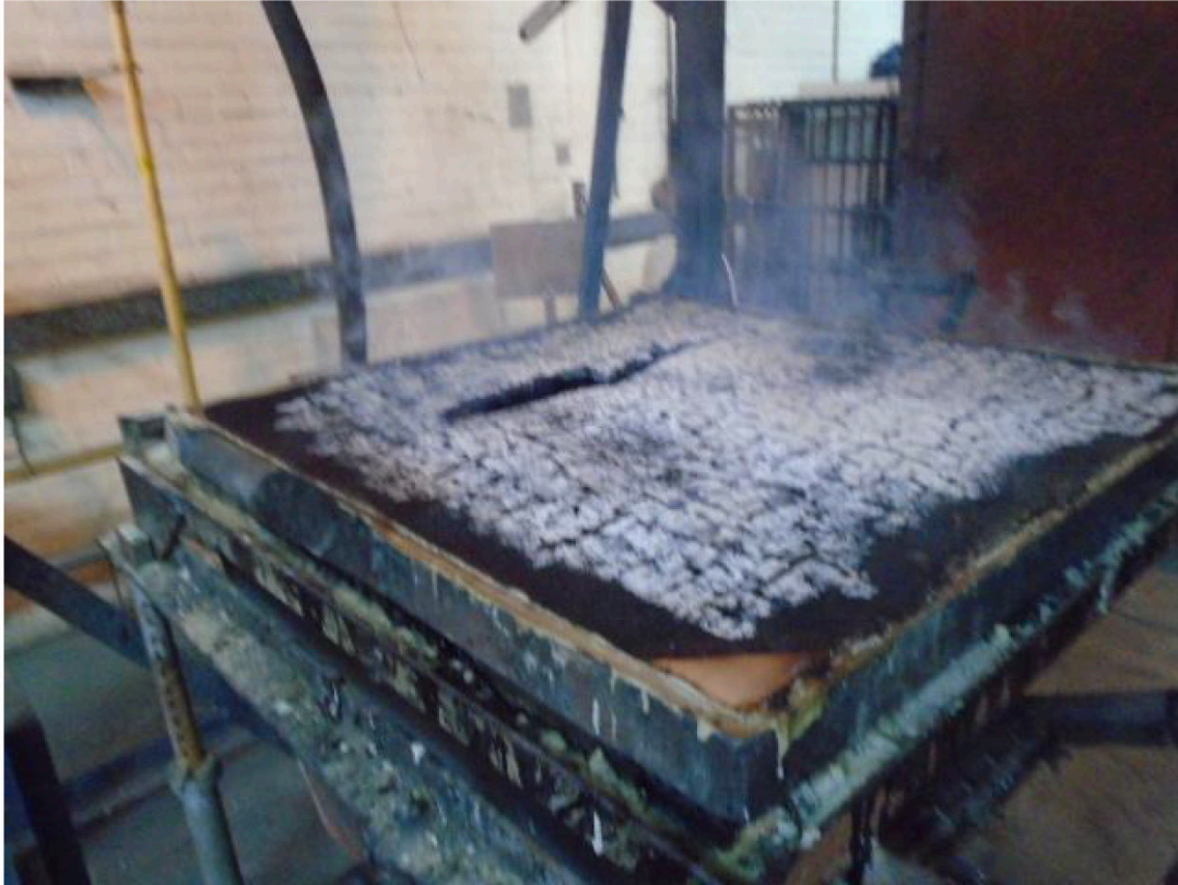
Figure 9- showing the failure at 40 minutes.
