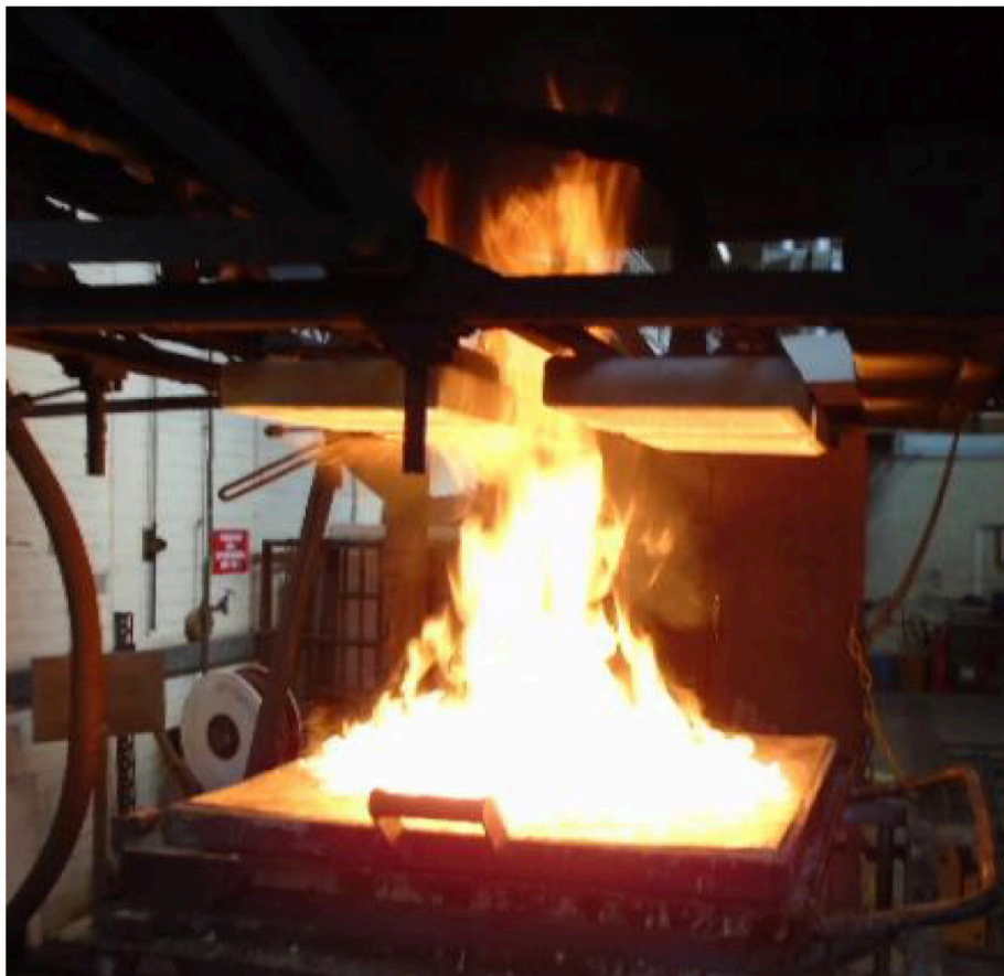
Figure 17- Test 2 immediately before test stopped at 7:00 minutes due to flames threatening gas pipes above test rig.
